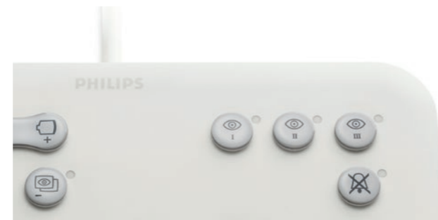
Figure 14: Position and labeling of the three fluoroscopy flavors on the user interface of the AlluraClarity and Allura Xper systems
